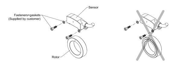
9. 3 B magnetic rotor - (Installation direction) The installation position of the rotor and sensor must not be changed! (As shown below)
